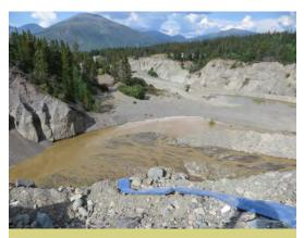
Sediment-laden water flowing from a placer mine site. These sediments can carry contaminants, such as aluminum, arsenic, and chromium—sometimes in levels that exceed drinking water standards.
